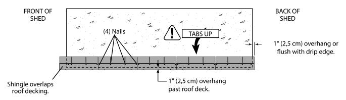
Beginning at front of shed, install first row of shingles with notch at 1" past roof edge or flush with drip edge.
