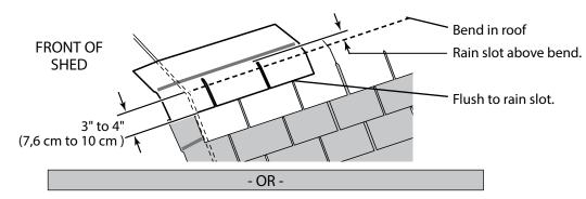
• If the rain slot of the shingle installed over the bend is BELOW the bend, install the shingle over the bend and overlap the rain slot to get the 3" to 4" overlap.
