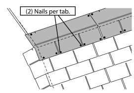
7 Continue installing rows of shingles to the peak. At the peak make sure there is a maximum of 5" or less to the rain slot, as shown below. If shingles overlap at ridge cut to peak with a utility knife.
