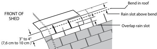
The shingle OVER the bend must be installed with a 3" to 4" overlap AND the rain slot above the bend.
