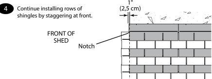
The shingle over the bend in the roof will be nailed down. You will need 3" to 4" of this shingle to extend downward over the bend for nailing.
