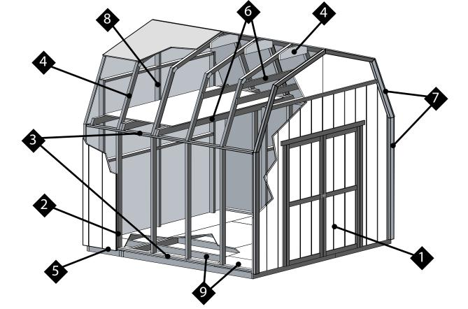
This building has been designed using our patented EZ Frame construction method. EZ Frame is a unique construction method which has been engineered to use fewer framing members. This reduces assembly time and cost by as much as 30% compared to conventional construction methods. EZ Frame patent no. 5,666,766
