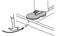
**3** Orient parts on edge. Use two 3" nails at each location.
