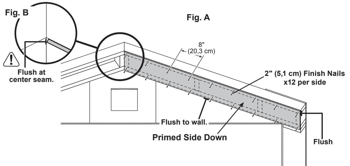
**2** Position left 73-5/16" overhang board **Primed Side Down** flush to front wall (**Fig C**), gable end and right overhang board (**Fig. D**). Secure using twelve 2" finish nails.
