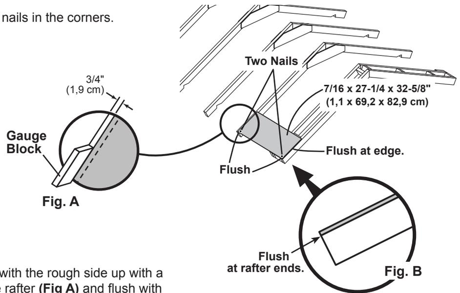
**2** Attach a 27-1/4" x 96" roof panel with the rough side up with a 3/4" (1,9 cm) measurement on the rafter (**Fig A**) and flush with the installed panel (**Fig. C**).
