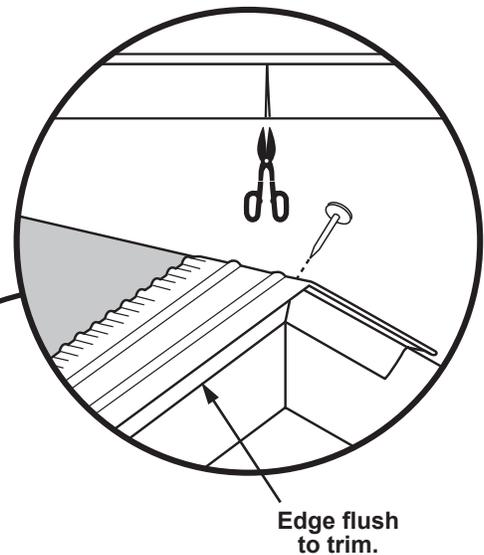
Snip bottom side of drip edge and bend over to other side of roof.
